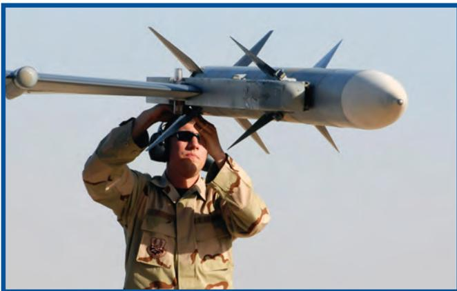
*Airman 1st Class Mark Drennen checks an AIM-120 missile on an F-16 Fighting Falcon.*
