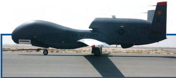
*A Global Hawk unmanned system vehicle is towed back to its hangar following a mission at a deployed location in Southwest Asia. Once mission parameters are programmed into a Global Hawk, the UAS can autonomously taxi, take off, fly, remain on station capturing imagery, return and land. Ground-based operators monitor the UAS's status, and can change navigation and sensor plans during flight as necessary.*
