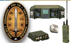
The LR is a handheld radio that connects Soldiers at the lowest echelon of the Army network by providing one-channel secure voice and data communications using Soldier Radio Waveform (SRW). The LR will simultaneously support Single Channel Ground and Airborne Radio System (SINCGARS) voice interoperability and Soldier Radio Waveform (SRW) data and voice communications in one radio with both dismounted and mounted configurations.
