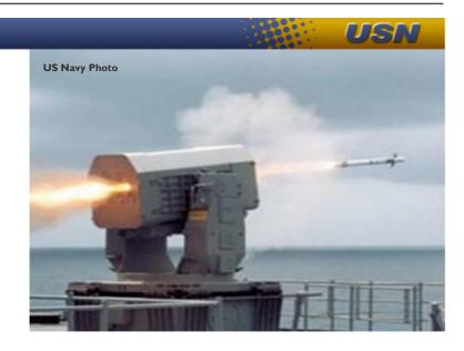
Infrared (IR) guidance for terminal engagement. Currently there are two RIM-116 configurations: Block I (RIM-116B) and Block II (RIM-116C).
