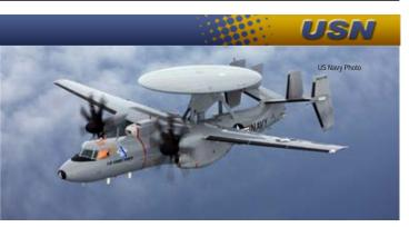
littorals; supports the Theater Air and Missile Defense operations; and improves operational availability for the radar system. Relative to the E-2C aircraft, the E-2D aircraft provides increased electrical power, a strengthened fuselage, and upgraded radar system, communications suite, and mission computer.
