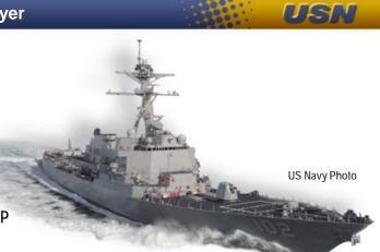
with a ballistic missile defense capability. The Arleigh Burke class is comprised of four separate variants; DDG 51-71 represent the original design, designated Flight I ships, and are being modernized to current capability standards; DDG 72-78 are Flight II ships; DDG 79-124 and DDG 127 ships are Flight IIA ships; DDG 125, DDG 126, and DDG 128-140 will be constructed as Flight III ships with the Air and Missile Defense Radar (AMDR) capability.
