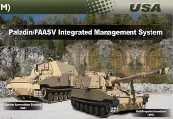
through 2050. The PIM replaces the current M109A6 Paladin and M992A2 FAASV vehicles with a more robust platform, incorporating the M2 Bradley common drive train and suspension components. The PIM fills the capability gap created by cancellation of the Non-Line of Sight Cannon (NLOS-C), a component of the Future Combat System program in 2009. Began Full Rate Production (FRP) in FY 2018.
