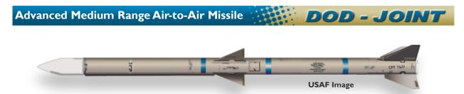
The Advanced Medium Range Air-to-Air Missile (AMRAAM) is an all-weather, all-environment radar guided missile developed to improve capabilities against very low-altitude and highaltitude, high-speed targets in an electronic countermeasures environment. The AMRAAM is a joint Navy/Air Force program led by the Air Force.
