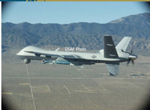
equipment; a support element; and trained personnel. The Reaper is a single-engine, turbo-prop, remotely piloted armed reconnaissance aircraft designed to operate over-the-horizon at medium altitude for long endurance.
