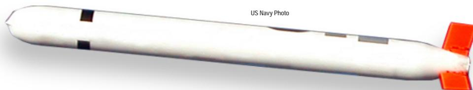
Tomahawk is a long range cruise missile used for deep land-attack strike warfare that is launched from U.S. Navy surface combatants and submarines. Tomahawk Block IV features an improved navigation/guidance computer; robust anti-jam Global Positioning System (GPS) capabilities; increased responsiveness and flexibility via satellite communications for in-flight re-targeting; a loiter capability; and the ability to transmit a Battle Damage Indication (BDI) prior to impact.
