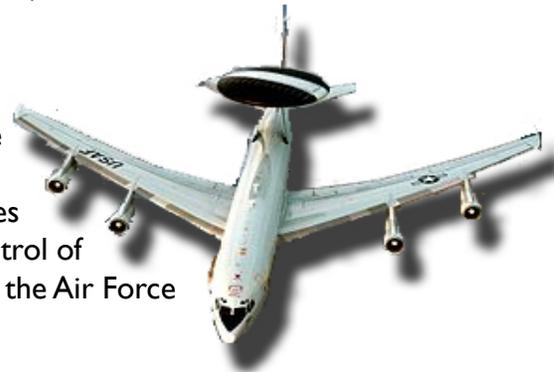
**Mission:** Provides surveillance, command and control (C2), and Communications functions for tactical and defensive missions.
