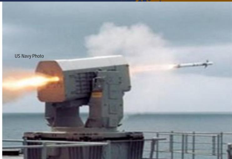
**Mission:** Provides high firepower close-in defense of combatant and auxiliary ships by utilizing a dual mode, passive radio frequency/infrared missile in a compact 21 missile launcher.
