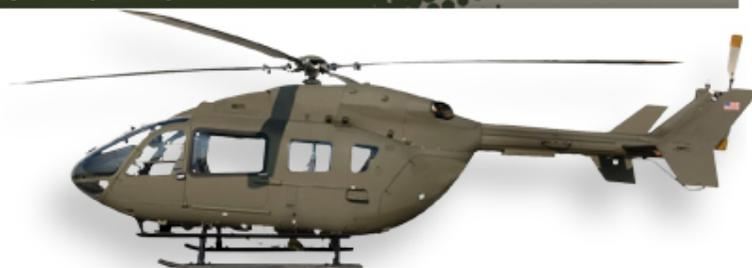
The UH-72A Lakota, which entered service in 2006, is a militarized version of the Eurocopter EC145 modified to an LUH configuration. It provides reliable and sustainable general and administrative support in permissive environments at reduced acquisition and operating costs. The LUH acquisition strategy is based on the competitive procurement of a commercial-off-the-shelf, non-developmental aircraft. There is no more developmental funding required for this program.
