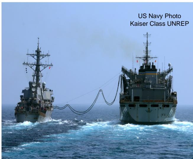
**Mission:** Transfers fuel to Navy surface ships operating at sea to extend at-sea time for the ships and embarked aircraft.
