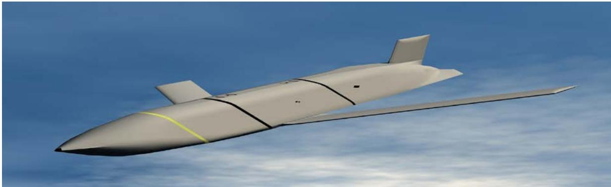
The Offensive Anti-Surface Warfare/Increment I develops the Long-Range Anti-Surface Warfare Missile (LRASM). LRASM is a precision-guided anti-ship missile with semi-autonomous guidance, day/night and all-weather capability. LRASM integrates a multi-modal sensor suite, a weapons data-link, enhanced digital anti-jam Global Positioning System capabilities, and a 1,000 lb penetrator/blast fragmentation warhead. OASuW/Increment I is a joint Navy/Air Force program led by the Navy.
