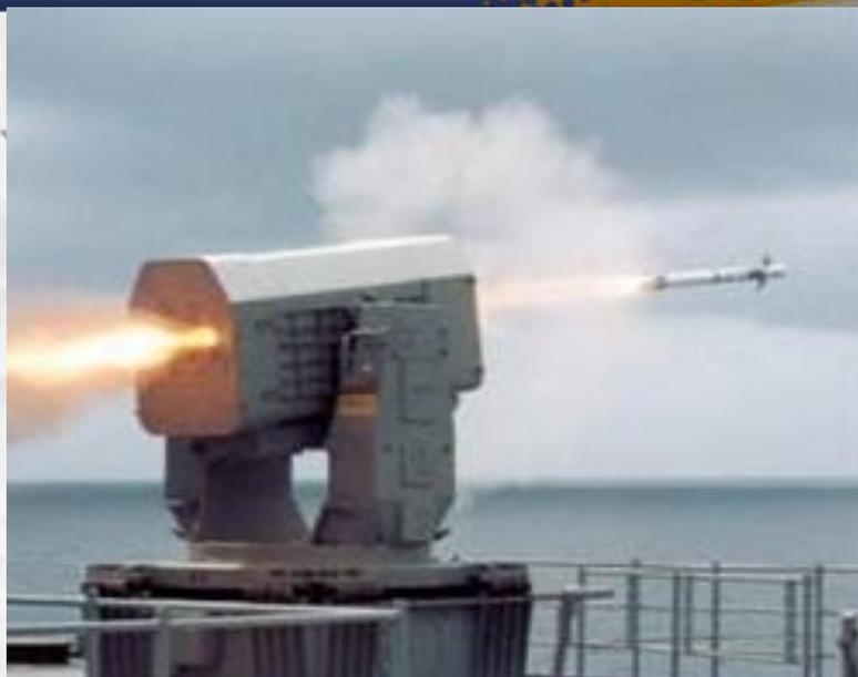
**Mission:** The mission of the RAM is to provide high firepower close-in defense of combatant and auxiliary ships by utilizing a dual mode, passive radio frequency/infrared missile in a compact 21 missile launcher.
