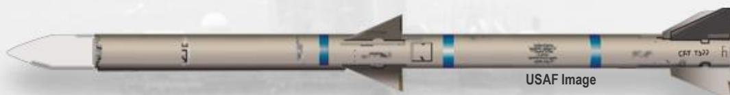
The Advanced Medium Range Air-to-Air Missile (AMRAAM) is an all-weather, all-environment radar guided missile developed to improve capabilities against very low-altitude and high-altitude, high-speed targets in an electronic countermeasures environment. The AMRAAM is a joint Navy/Air Force program led by the Air Force.
