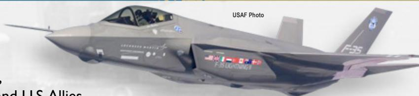
The JSF consists of three variants: Conventional Take-Off and Landing (CTOL), Short Take-Off and Vertical Landing (STOVL), and Carrier (CV).
