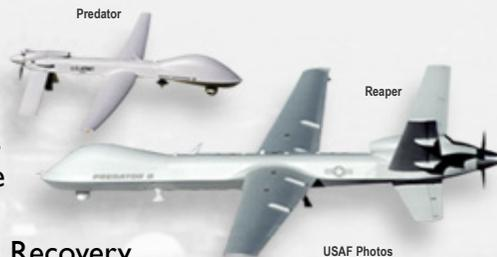
**Mission:** A single-engine, remotely piloted armed reconnaissance aircraft designed to operate over-the-horizon at medium altitude for long endurance. The primary mission is reconnaissance with an embedded strike capability against critical, perishable targets. The Army MQ-1C Gray Eagle also has the unique mission of communications relay.
