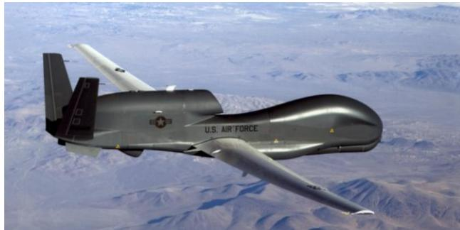
An RQ-4 Global Hawk soars through the skies in route to record intelligence, surveillance and reconnaissance data. Because of its large coverage area the Global Hawk has become a useful tool for recording data and sending it to warfighters on the ground.
