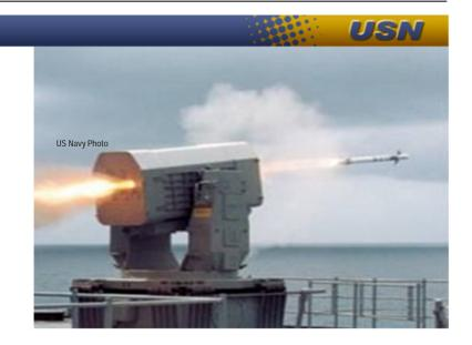
terminal engagement. Currently there are two RIM-116 configurations: Block I (RIM-116B) and Block 2 (RIM-116C).
