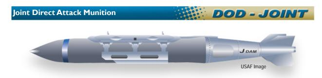
The Joint Direct Attack Munition (JDAM) is a joint Air Force and Navy program led by the Air Force. The JDAM improves the existing inventory of general purpose gravity bombs by integrating a Global Positioning System (GPS)/inertial navigation guidance capability that improves accuracy and adverse weather capability.
