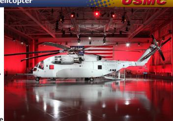
only heavy-lift platform that can lift the MAGTF ashore. It will provide an unparalleled high-altitude lift capability with nearly three times the external lift capacity of the CH-53E. A total of 194 aircraft are planned for procurement. First flight will be completed in FY 2015, and the program is working towards a Milestone C decision in FY 2016.
