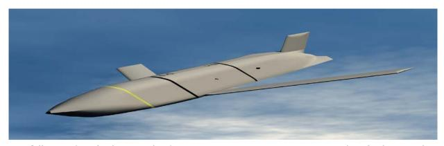
The Offensive Anti-Surface Warfare/Increment I develops the Long-Range Anti-Surface Warfare Missile (LRASM). LRASM is a precision-guided anti-ship missile with semi-autonomous guidance, day/night and all-weather capability. LRASM integrates a multi-modal sensor suite, a weapons data-link, enhanced digital anti-jam Global Positioning System capabilities, and a 1,000 lb penetrator/blast fragmentation warhead. OASuW/Increment I is a joint Navy/Air Force program led by the Navy.
