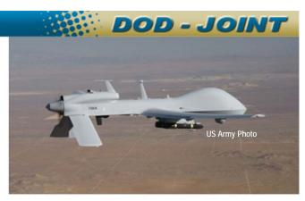
line-of-sight and beyond-line-of-sight control. Both systems include single-engine, propeller-driven unmanned aircraft.
