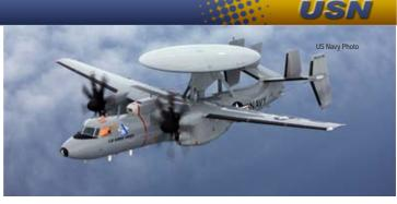
littorals; supports the Theater Air and Missile Defense operations; and improves operational availability for the radar system. Relative to the E-2C, this variant of the E-2 provides increased electrical power, a strengthened fuselage, and upgraded radar system, communications suite, and mission computer.
