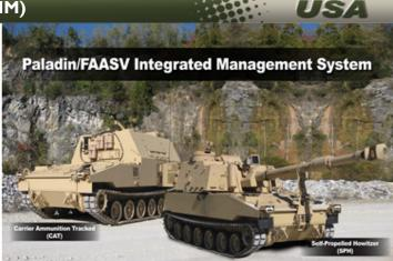
FOV through 2050. The PIM replaces the current M109A6 Paladin and M992A2 FAASV vehicles with a more robust platform, incorporating the M2 Bradley common drive train and suspension components. The PIM fills the capability gap created by cancellation of the Non-Line of Sight Cannon (NLOS-C) (a component of the Future Combat System program) in 2009. The PIM is in Low Rate Initial Production (LRIP).
