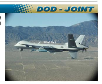
equipment; a support element; and trained personnel. The Reaper is a single-engine, turbo-prop, remotely piloted armed reconnaissance aircraft designed to operate over-the-horizon at medium altitude for long endurance.
