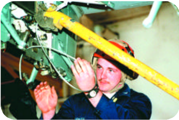
An Aviation Electronics Technician positions the cable that will hoist a MK62 mine onto the P-3's bomb rack at the Naval Air Station, Jacksonville.
