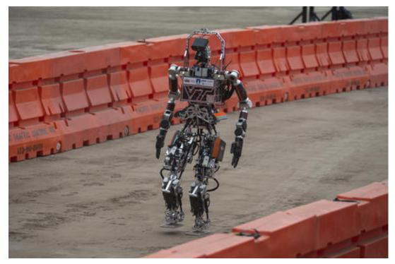
ESCHER, short for Electric Series Compliant Humanoid for Emergency Response, makes its way down the track during day two of the Defense Advanced Research Projects Agency Robotics Challenge (DRC). ESCHER was designed, fabricated, and assembled by engineering students at Virginia Tech.
